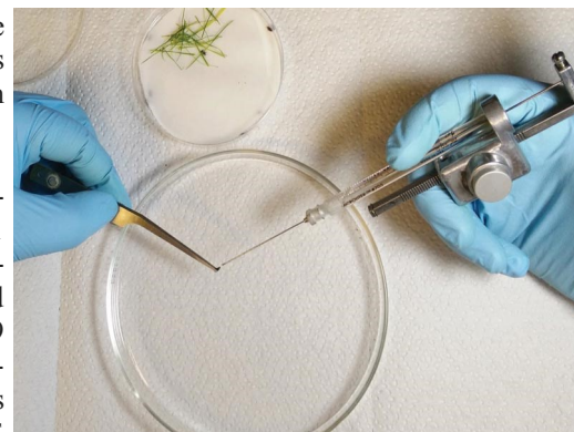
A microapplicator was used to apply the active ingredients of insecticides in the topical bioassays. Photos by Olga Kostromytska
